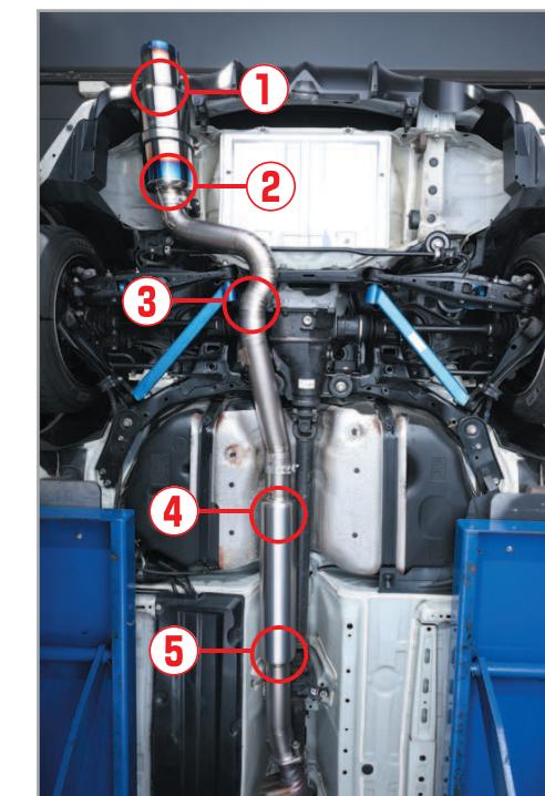
This new model from Ti RACING series was designed to overcome all the negative points the previous model of EXPREME Ti had. Higher flow along with improved ground clearance of +10mm at the diff cradle on ZN6/ZC6 where is the lowest point. (measurements from the chassis to each point)
