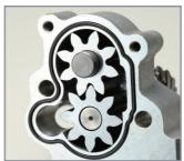
The thick 20mm gear significantly increases the flow rate.
