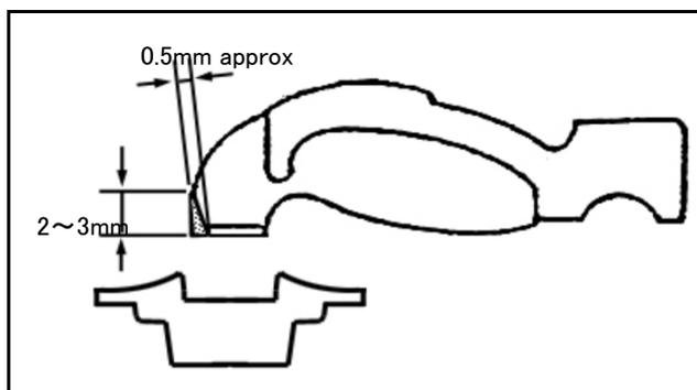
The retainers that are to be used on the Type B for SR20 can at times interfere with the rocker arms so depending on the application of the setup may require the rocker arm tip to be shaved about 1mm to allow appropriate clearance. Look at the illustration to the left for reference.
