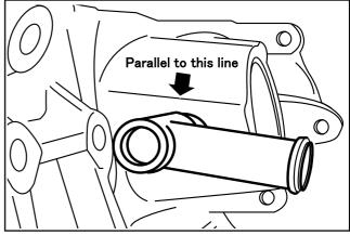
Do not hammer directly on the TOMEI Water Connector to prevent to damage the product when pressing in. XUse a soft-head hammer and or a metal sheet of soft metal such as aluminum or copper to prevent XUse a soft-head hammer and or a metal sheet of soft metal such as aluminum or copper to prevent damaging the product. Do not use excess force to install the product into the position.
