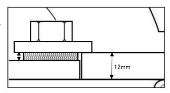
③ Ensure intake and exhaust manifolds are not interfered or touched each other. In the case they are interfered or touched, cut off the point little by little.
