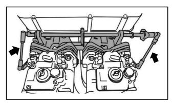
(2) Thickness of intake manifold flange is t=12mm. Adjust the thickness of exhaust manifold flange using washer to fasten down these 2 flanges together.
