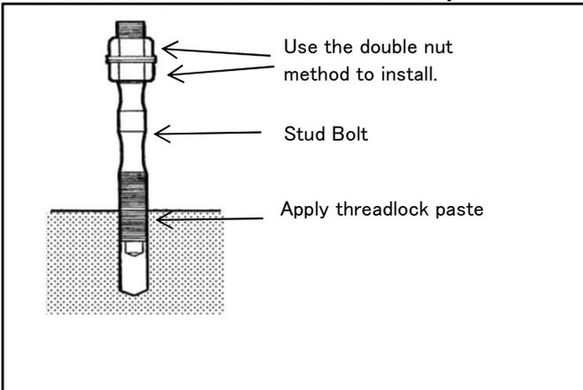
① Fit both nuts on the top of the stud, in the double nut arrangement.
