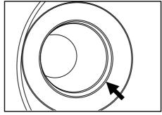
5. Check for any interference and tighten Clamp Band  $\phi$  80 to the specified torque.
