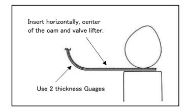
(3) Assemble with selected shims and measure all the clearance again. Repeat above procedures as needed.
