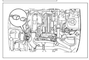
(1) Remove the Solenoid Valve Connector.
