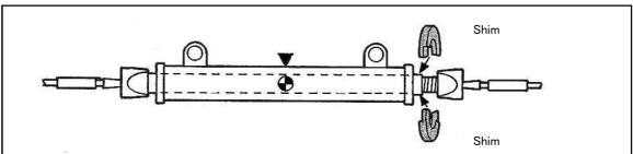
$\ensuremath{\mathfrak{G}}$  Secure the Shims in place with the Screws.
