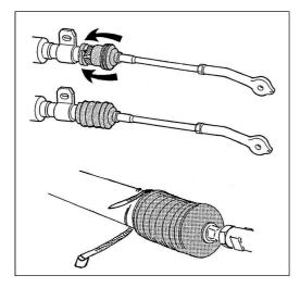
4 Fit the boots over the shim, and tie in place with the large cable tie.
