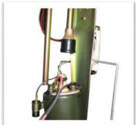
The original pump is only plugged into the unit. Pull straight out the original pump.
