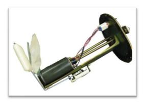
Carefully remove the fuel sender unit assembly from the gas tank not to get the level sensor float caught by the edge of the gas tank hole that may damage or bend the level sensor float/arm.
