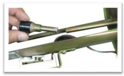
Attach the Pump Bottom Isolator to TOMEI Fuel Pump, mount it on the fuel sender unit using the pump retainer. Then mark on the metal pipe of the fuel sender unit at where the Fuel Hose reaches, then go down more than 20mm from the mark and make another marking. Cut off the metal pipe at the second marking point.
