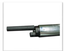
Install the Fuel Strainer to TOMEI Fuel Pump using the Mounting Clip.
