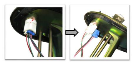
Disconnect the blue wire connector from the fuel sender assembly.
