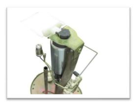
Verify the fuel sender unit is assembled properly and tighten the Hose Clamps securely.
