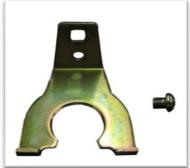
Remove the bolt of the retainer that secures the fuel pump to the fuel sender assembly.
