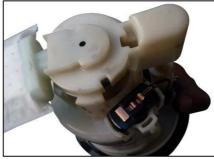
Attach the rubber isolator that was removed from the bottom of the stock pump earlier, and put the plastic bottom cover back on the fuel sender unit assembly.
