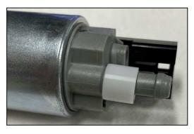
Slide in the kit-included Spacer Collar onto the outlet port of TOMEI Fuel Pump.
