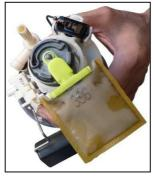
Remove the bottom cover of the fuel sender unit by releasing the latches, be careful not to break them. (NOTE: Keep the rubber isolator attached to the bottom of the pump body, it will be reused later.)
