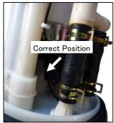
Connect the wiring harness to TOMEI Fuel Pump and put it back into the fuel sender unit.
