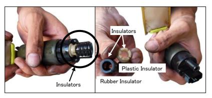
Remove the insulators from the outlet port of the stock pump.
