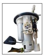
Carefully remove the fuel sender unit assembly from the gas tank not to get the level sensor float caught by the edge of the gas tank hole that may damage or bend the level sensor float/arm.
