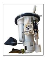
Remove the fuel pump from the fuel tank. Take care not to get the float stuck so as not to damage or break it.
