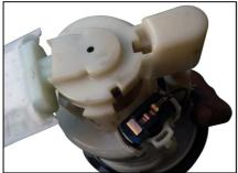
The insulator which was first removed from the fuel pump, is now to be fitted back onto the pump. Fit the cover back onto the assembly.
