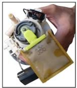
Remove the fuel pump units cover. Work with care so as not to break or damage anything.
