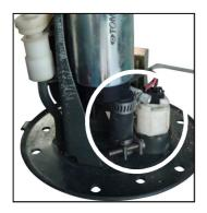
Connect the coupler to the fuel pump body, then the fuel hose to the bracket.
