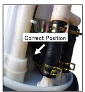
The coupler is connected to the fuel pump, the fuel pump is inserted in pump assembly.
