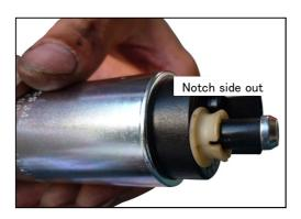
The insulator which was removed earlier, is now to be fitted to the mouth piece of the fuel pump.
