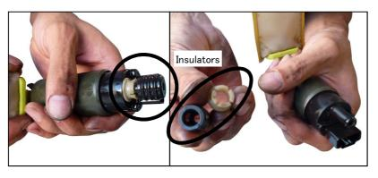
Remove the insulator which was on the pump. (Keep them to re-use it later)
