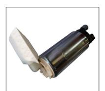
Fit the filter to the fuel pump (included).
