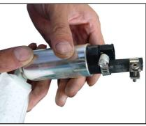
Fit the fuel filter to the pump with the clip (included). Then fit the hose clamps over the hose before installing the cut fuel hose to the pump.
