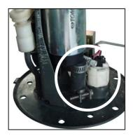
Connect the coupler to the fuel pump body, then the fuel hose to the bracket.
