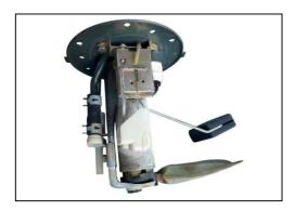
Remove the fuel pump from the fuel tank. Take care not to get the float stuck so as not to damage or break it.
