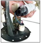
Loosen the band on the bracket side of the fuel hose.
