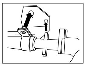
(2) Place the hose-to-strainer fitting to fit in the notch on the bracket, then tighten them together using the kit-included M4 Bolt and Square Nut.
