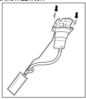
(1) Build the TOMEI Fuel Pump onto the fuel pump bracket and fix in place with the 2 clips removed earlier.
