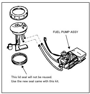
(1) Disassemble the fuel sender unit assembly and remove the fuel pump assembly from the unit.
