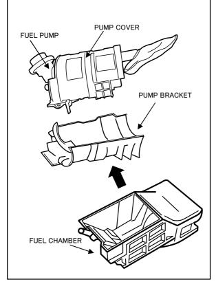
(2) Remove the stock fuel pump body from the fuel pump assembly, then also the pump cover and the pump bracket.
