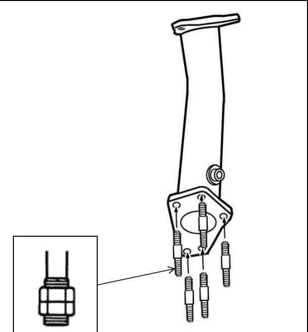
※ Be careful not to loosen the stud bolt when removing the double nut.
