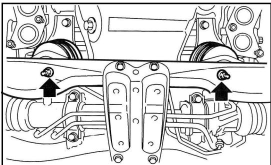
It may not separate well with vehicles according to the clearance condition of a support pipe and a member at the time of support pipe removal.
