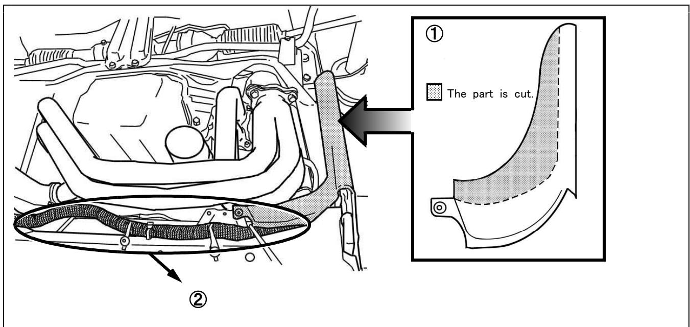
① Cut the undercover at manifold area, as shown in the above figure.
