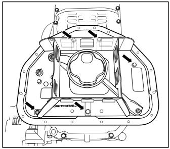
5. Check for interference between the Lower Baffle and the stock oil pan.
