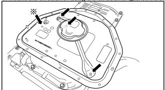
⚠ Lightly tighten the 4 bolts marked as X in the left, just enough to fit everything up in place at this point.
