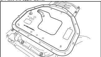
3. Mount the oil strainer using the oil strainer gasket included in the kit.
