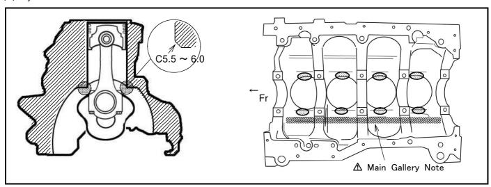
The points to take note of are the 8 points located at the bottom of the cylinder walls in which will interfere with the conrods. Adjustments are required to allow 1mm to 1.5mm of clearance which can be made with a hand router or other specialized milling tools.
