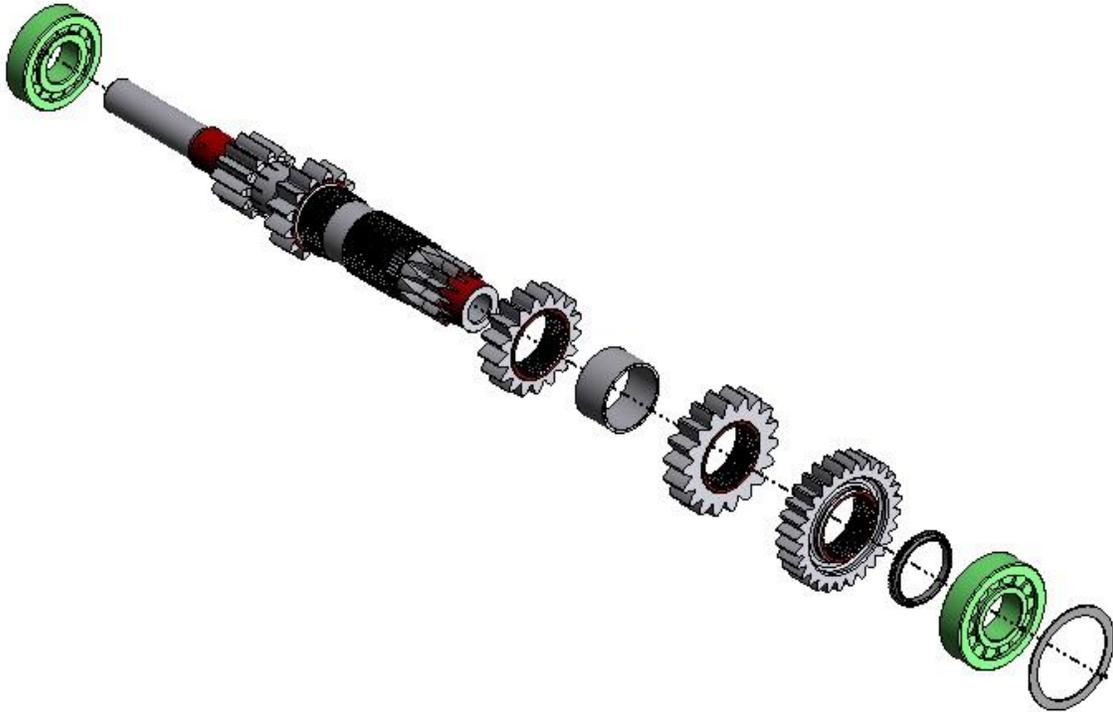
Start by sliding the 3<sup>rd</sup> Spline-Gear onto the shaft and up against the integral 2<sup>nd</sup> Gear. Follow this with the 3<sup>rd</sup> /4<sup>th</sup> Input Shaft Spacer (*HLE-102*), then 4<sup>th</sup> and 5<sup>th</sup> Spline-Gears.
