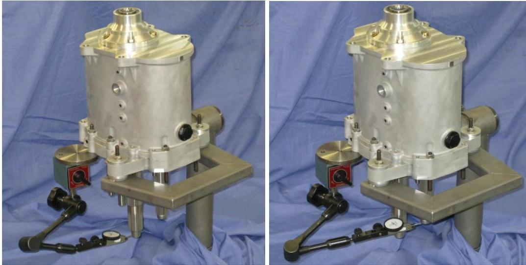
Grind and fit new shims to set the end float between 0.003"-0.005" (0.075mm-0.13mm) for both the Mainshaft and Layshaft.
