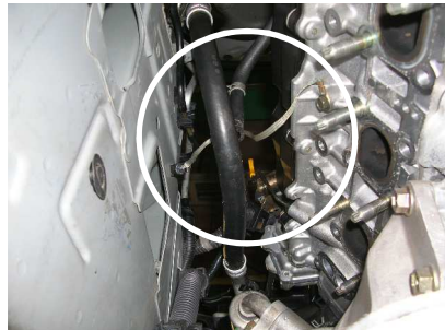
On the left side of the car is the body earth
