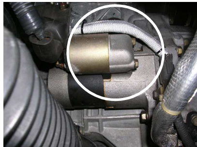
Starter Motor wiring on the car bodys left side
