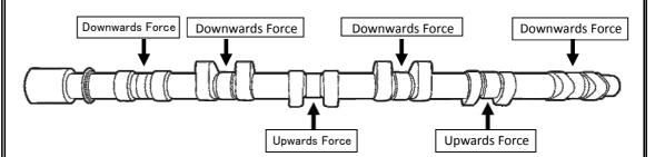
When tightening the cam journals, you'll have to pay attention to the direction of the lobes. Try to sink the cam slowly into the head as verticle as possible, doing up each screw slowly each time until the cam is sitting safetly in position before finally tightening it all into place.
