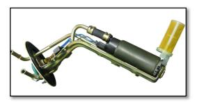
Carefully remove the fuel sender unit assembly from the gas tank not to get the level sensor float caught by the edge of the gas tank hole that may damage or bend the level sensor float/arm.
