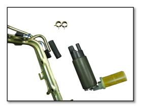
Remove the fuel hose from the fuel sender assembly.
