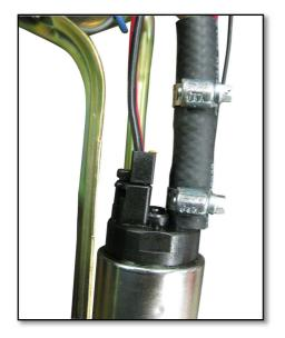
Tighten the Hose Clamp at the pump side securely, then connect the Wiring Harness to the TOMEI Fuel Pump.
