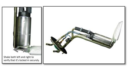
Again, verify that the fuel pump is properly and securely fixed on the fuel sender unit in it's position. Then install the fuel sender unit assembly back into the gas tank.
