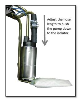
Connect the Fuel Pump to the Fuel Hose pre-assembled on the fuel sender unit, then place the Pump Bottom Isolator securely.
