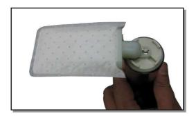
Install the Fuel Strainer to the TOMEI Fuel Pump using the kit-included Mounting Clip.
