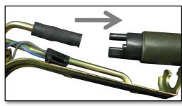
Disconnect the fuel hose from the pump body..
