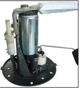
Put back the brackets and the fastener the same as before. Fit the kit-included Rubber Bottom Isolator.
