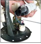
Loosen the hose clamp on the bracket side of the fuel hose.
