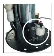
Connect the wire connector to the TOMEI Fuel Pump body, then the fuel hose to the bracket.
