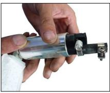
Fit the Strainer to the pump with the kit-included Clip. Then fit the kit-included Hose Clamp over the hose before installing the cut fuel hose to the pump. Then tighten the Hose Clamp in place on the pump side.
