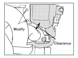
Please ensure that there is adequate clearance between the blow-by separator and the exhaust manifold 4th pipe. If there is inadequate clearance you can increase the size of the mounting holes so you can adjust the position to have adequate clearance.
