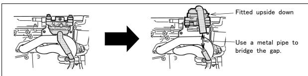
•When the EAI Control Valve is fitted upside down the hose will require an additional metal pipe to be able to reconnect it. This metal pipe is also available separately as an option (Part Number: 191232).
