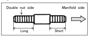
2 The stud bolts are then fitted on teh exhaust manifold
