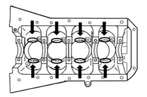
The marked areas as shown on the illustration on the left, shows areas where the Conrods may make contact when changing the cylinder sleeves.
