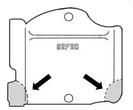
Cut away the 2 end bits as shown on the illustration on the left.
