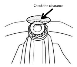
The marked areas as shown on the illustration on the above,conrods may make contact. (Where the 50mm~65mm away from the matching surface of oil pan/block)
