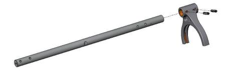
Place the 5<sup>th</sup>/6<sup>th</sup> Fork (*HTA-025*) on the *RD6-074* Selector Rod as shown.
