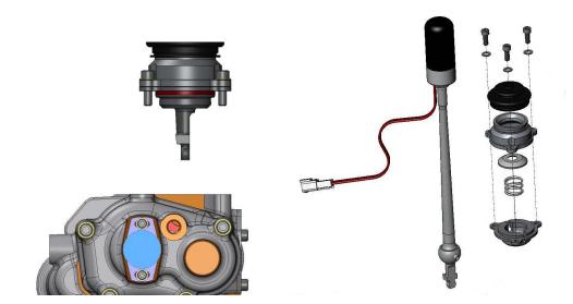
NOTE: If the gearbox is a remote-shift version, ignore the last step and install the *H6S-142* Selector Housing Cover and secure with *M6x12mm Cap Screws* and sealant. Then install the Remote Clevis *H6S-SEQR-017* securing with a 5x19mm Roll Pin.
