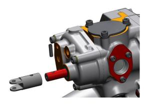
The Detent Plunger (*H6S-SEQ-014*), Detent Spring (*H6S-027*) and Plug (*RD6-122*) must now be installed and secured using Loctite 243 (blue). Tighten to 15FtLb (20Nm).
