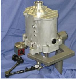
Grind and fit new shims to set the end float between 0.003"-0.005" (0.075mm-0.13mm) for both the Mainshaft and Layshaft.
