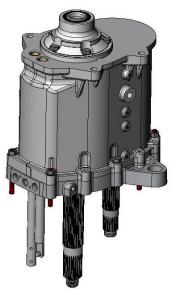
Use a dial indicator check the end float on the shafts.
