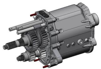
TIP: Visually check the gear tooth backlash to be 0.008" (0.2mm), Also check the gear end float to be 0.009"-0.012"
