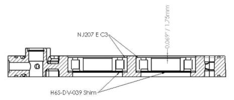
cross section view of sandwich plate
