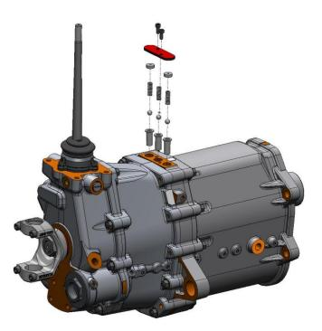
Insert three lubricated GRA-6N-036 detent sleeves into the sandwich plate followed be 5/16" balls, GRA-6N-080 Detent springs and HTA-046 Detents spacers in the outer two detent bores. Attach using two M5x12mm SHCS, using sealant on the GRA-6N-060 spring plate.
