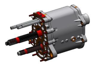
Next remove the front cover, which is held on by five M8 bolts. Locate the end float shim (H6S-DV-040) from in front of the input bearing.
