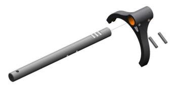
Place  $1^{st}/2^{nd}$  fork (HTA-025) on RD6-006 selector rod as shown. Secure the forks onto the selector rods with 5mm x 22mm roll pins.
