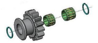
Insert a 140-20 (BR20) circlip into one side of the RD6-130 reverse idler. Place both bearings 106-162013, and 106-162017, into the bore of the gear and retain them with a second circlip.
