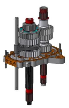
Then fit the 5<sup>th</sup>/6<sup>th</sup> selector ring and selector fork/rod.
