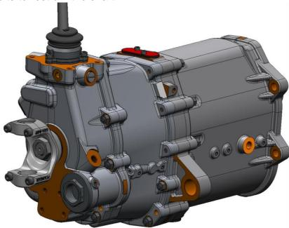
Now you can install the Selector housing cup, Gear lever, spring, washer, cap and rubber boot using 3, M6x16mm SHCS.
