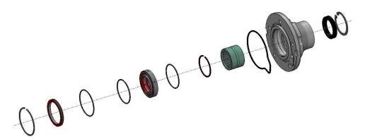
Warm the RD6-150 cover until the 108-354530 (NK35/50) bearing slides into position. Then retain the bearing with a 140-45 (BR45) circlip. Ensure the position of the circlip allows for easy removal.
