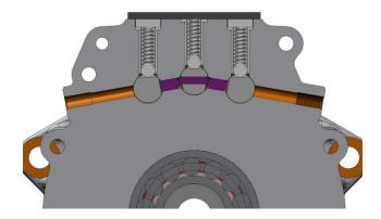
Check the interlock pin RD6-024 is fitted in the  $3^{rd} / 4^{th}$  selector rod. Then install the mainshaft, together with the  $3^{rd}/4^{th}$  selector fork/rod and the layshaft as per diagram. Move the  $3^{rd}/4^{th}$  fork and rod into its neutral position so that the interlock plungers allow  $5^{th}/6^{th}$  to be fitted in the next step.
