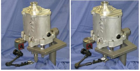
Grind and fit new shims to set the end float between 0.003"-0.005" (0.075mm-0.13mm) for both the main and layshafts.
