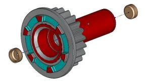
Two Welch plugs are fitted to the input shaft. The front plug is unmodified. The rear (dog end) plug requires a 3mm hole in its centre, to form the oil jet.
