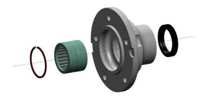
Assemble the front cover as mentioned above, however it will require sealant on its mating surface once assembled onto the front case as is does not have an O-Ring to seal.
