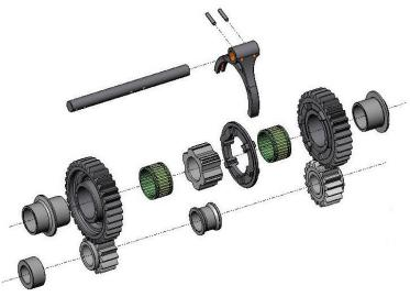
Place 106-424727 needle rollers onto the two remaining bearing sleeves, RD6-160, and RD6-161. Lubricate them with gear oil and place the 1<sup>st</sup> dog (2<sup>nd</sup> if O.D.) gear onto the RD6-161 sleeve, and the 2<sup>nd</sup> dog gear (1<sup>st</sup> if O.D.) onto RD6-160 sleeve.
