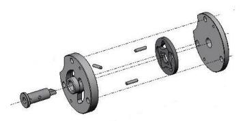
Insert the RD6-020 oil pump spindle into the RD6-022 pump housing, then place a 3x15.8mm roll through the exposed hole in the spindle.
