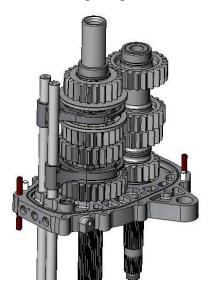
Grease the dowels, and place the maincase over this assembly. Make sure the selector rods can travel freely and the shafts turn freely.
