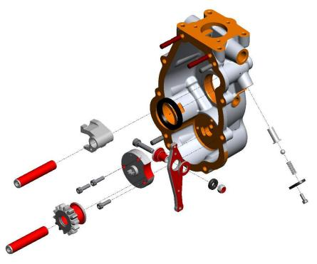
Lubricate and place the oil pump assembly into the base of the casting and secure with M6x20mm cap screws. Retain the screws with lock wire.
