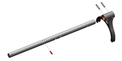
Place the  $3^{rd}/4^{th}$  fork (HTA-025) on the RD6-007 selector rod as shown, then slide the RD6-024 interlock pin into the small hole with grease.
