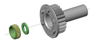
Place the input shaft on top of mainshaft assembly. Then fit the drop gear to the layshaft, followed by the H6S-DV-044 shim and the layshaft front bearing inner race. According to the following diagram:
