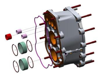
Insert two 120-1620DU bushes in through the rear of the case. Tap them into place so the two outer bushes sit just below the rear surface. Then insert one 120-2220DU bush into the centre of the case, until it is flush with the surface.
