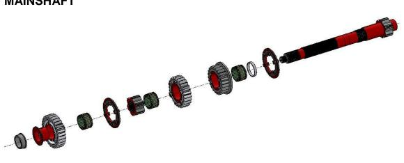
Start by sliding the bearing spacer and needle rollers up against the integral hub. Generously lubricate them with gear oil. The spacer must be beneath the integral dog on  $5^{\text{th}}$  (6<sup>th</sup> if overdrive).
