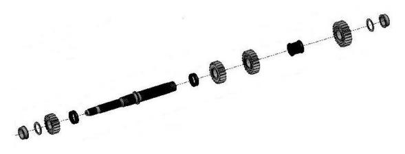
Begin by sliding an HTA-057 spacer, the 3<sup>rd</sup> spline gear (4<sup>th</sup> if O.D.), and the HTA-075 spacer onto the rear of the layshaft as shown in the left side of the diagram.
