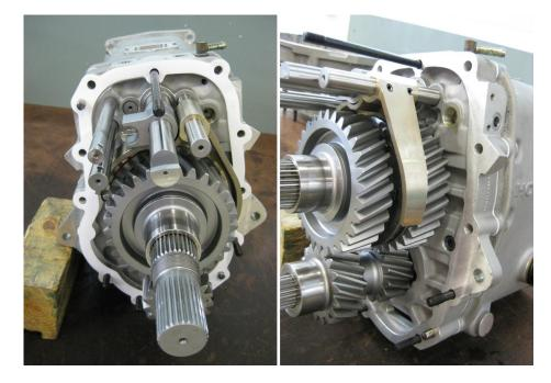
Remove 1<sup>st</sup> and 2<sup>nd</sup> Gears/Spacers/Sleeves, along with the Selector Ring/Hub and Rod/Fork.
