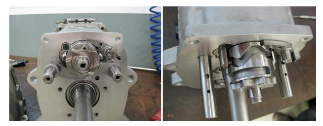
Remove the Camshaft by pulling it away from the rest of the gearbox.
