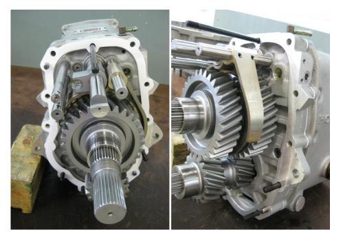
Now install the Rear Case. Whilst installing the Rear Case the Gear Lever Rod must be connected to the Intermediate Rod by the use of the Rod Connector, then the Neutral Actuator must slide over the connector. The Striker must also be placed onto the Neutral Latch Rod, whilst sliding the Rear Case Forward.
