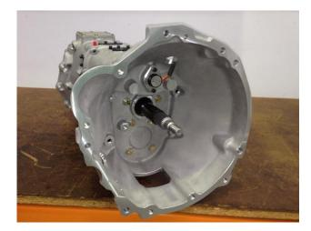
Begin by removing the 4 x M12 nuts/Washers. Then remove the Detent plunger and Spring which is located on the upper left side of the Bellhousing, under the black plug.
