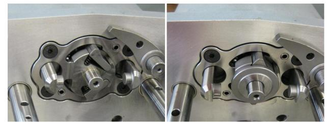
Now fit the Camshaft, 3<sup>rd</sup>/4<sup>th</sup> Cam Follower, Reverse Cam Follower, Neutral Lockout Spring and Washer:
