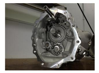
Select either 3<sup>rd</sup> or 4<sup>th</sup> gear by moving the selector rod protruding from the front of the gearbox, and simultaneously select Reverse gear by moving the other protruding rod (This locks the gearboxes shafts together allowing the rear nut/bolt to be removed).
