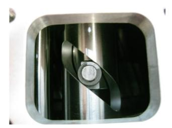
NOTE: It may be helpful to try and support the pin on the under-side to remove the Circlip/Washer/Rollers from the top. If the gearbox is being completely disassembled do not worry if the parts fall into the gear train, so long as they are retrieved after the Maincase is removed.
