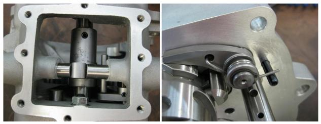
Now the cast Rear Cover can be placed over the plungers. Make sure it is sealed with an appropriate sealer.
