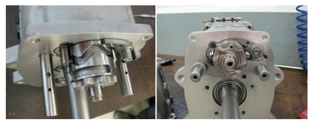
NOTE: If installing a new Camshaft or Bearing the Shim underneath it may need to be adjusted. Please contact Holinger directly to receive proper instruction on how to calculate the required thickness.
