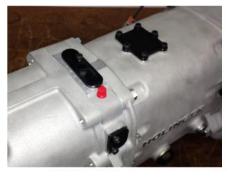
NOTE: The plates located on the sandwich plate will release Detent Springs/Balls. Be Careful not to lose them!
