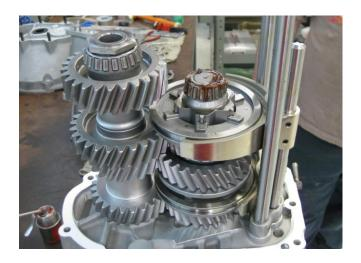
NOTE: Before installing the Input Shaft, ensure that the Pocket Bearing is well lubricated with Oil/Grease!
