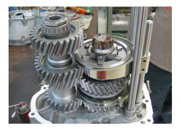
You can now remove all the parts, starting with the Input Shaft, then the Layshaft, the Mainshaft and Selector Forks/Rods.
