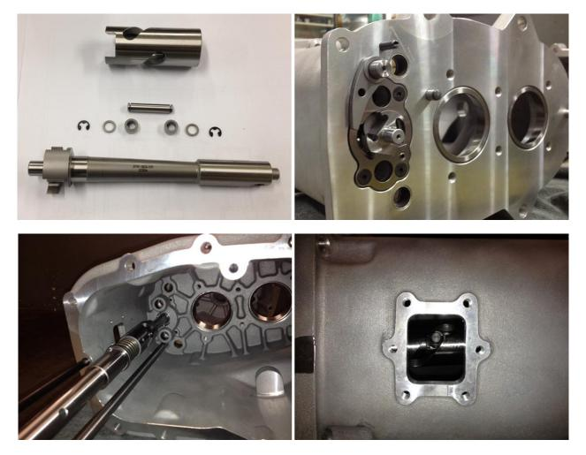
Place a new Gasket onto the Sandwich Plate then lower the Maincase over the assembly. Lightly tap it home with a soft hammer ensuring it goes on square and even onto the locating Dowels.
