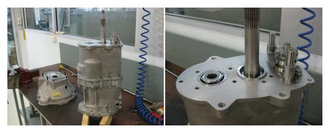
Knock the Rollpins out from the 3<sup>rd</sup>/4<sup>th</sup> and Reverse Cam Followers, and remove them from the selector rods. You can now also remove the Circlip/Washer/Spring from the Neutral Lockout Latch.
